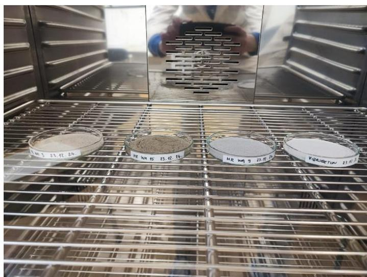
**Figure 12.** Samples inside a carbonation chamber
