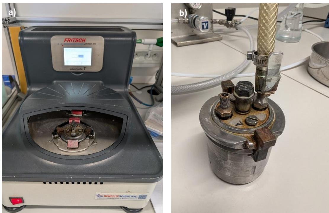
**Figure 14.** a) Planetary ball mill; b) Grinding jar equipped with a gassing lid for CO<sub>2</sub> pressurization
