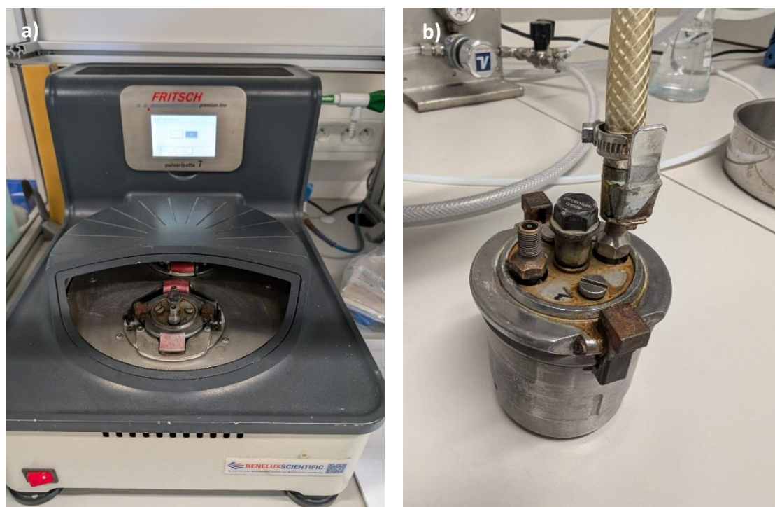
Figure 3. a) Planetary ball mill; b) Grinding jar equipped with a gassing lid for CO 2 pressurization
